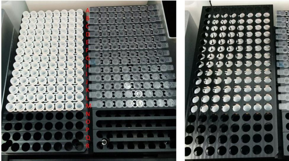
10. Place the qPCR reagents into the designated position of the rack.
