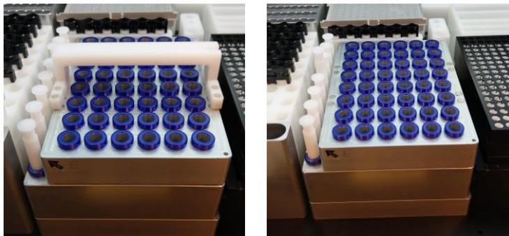
**“Elution cover on wrong direction, put it on elution manifold correctly ”**
