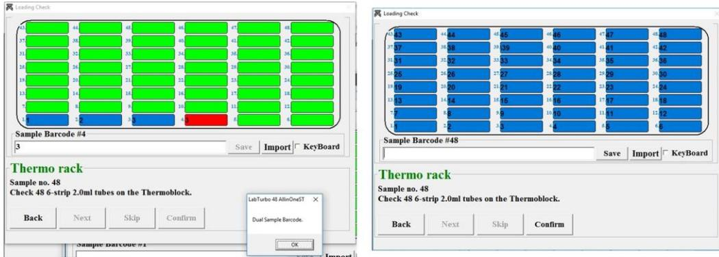
B. For elution tube barcode recording, please select “barcode” before tapping the elution tube section on the screen. The barcode input sheet will display. Follow the highlight in the **yellow** to scan the associated barcode on each elution tube. Once a barcode is keyed in and matched, it will be marked in **blue**. To modify the barcode, select the barcode to be modified and key in the correct barcode.
