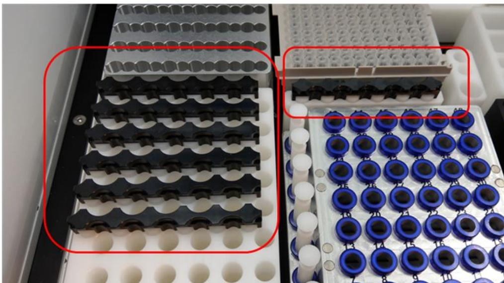
3. Put **Plug tubes** back to the **Plug tube rack**.
