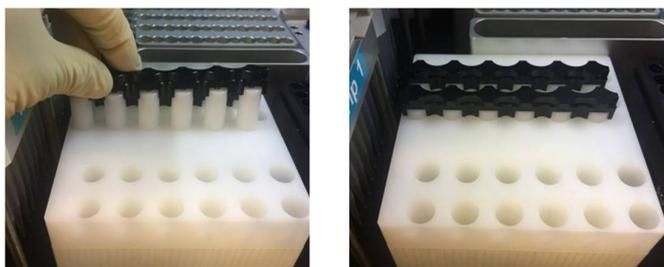
4. Put **Plug tubes** back to the **Plug tube rack**.
