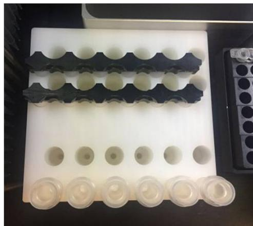
This message also indicates the **Plugset** is at the incorrect position. For example, six plugsets are set at the incorrect positions on the left picture. Please refer to the **Monthly clean and maintenance** section (section 7.3) for the plugset setup instruction.
