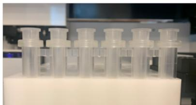
9. Put eppendorfs into the rack of **Elution vacuum manifold**.
