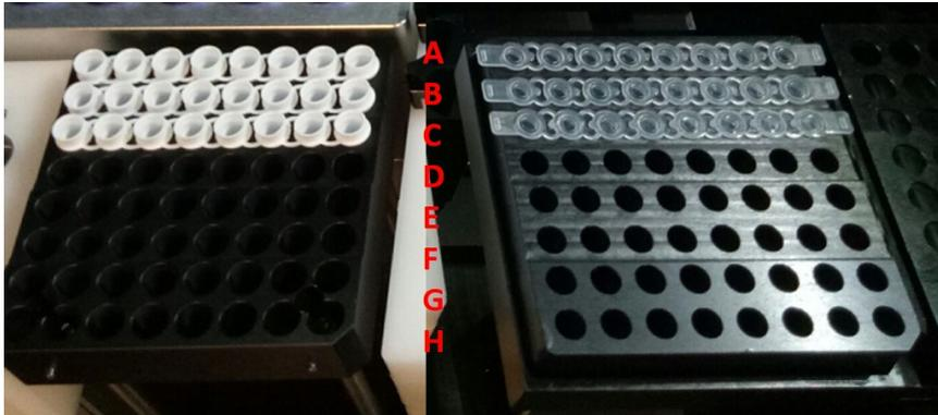
11. Place the qPCR reagents into the designated position of the rack.
