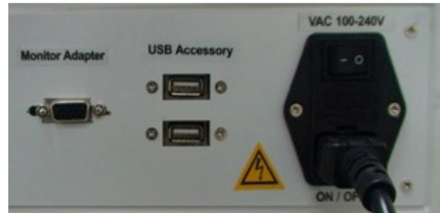
C. AC 110V/220V and ON/OFF are the main power switch and the power cord socket. The fuse chamber is in between the main power switch and the power cord socket.
